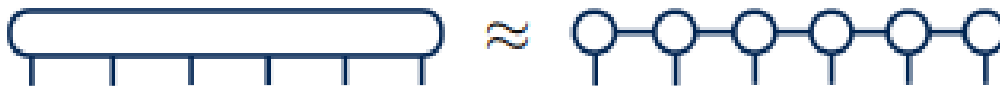
Figure 1: MPS decomposition, also known as a tensor train. (Lines represent tensor indices and connecting two lines implies summation)
