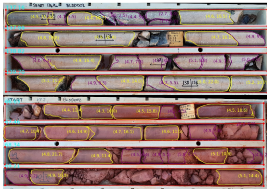
Figure: Example rock segmentation and measurement used to produce rock quality designation RQD from core photographs. The model is trained to predict the boundaries of rock fragments and measure them (e.g. 4.7, 10.4 = 4.7 cm high and 10.4 cm long). Yellow colours represent rock fragments larger than 10 cm long, blue segments are less than 10 cm long.
